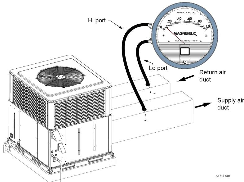
To measure the external static pressure, do the following:
