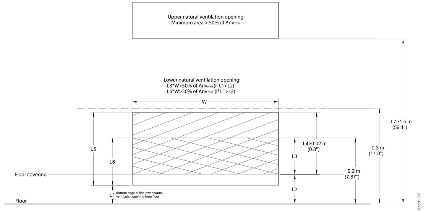
**Figure 2: Natural ventilation openings - lower opening partially below the 0.3 m point above the floor**
