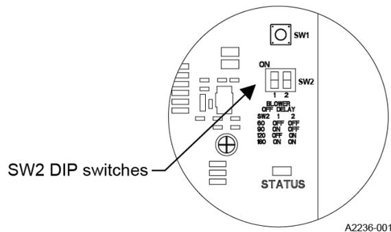
To configure the gas heating blower off delay settings, do the following:
